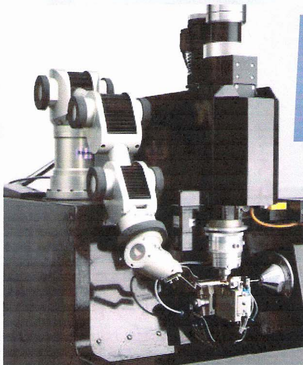
FIGURE 2. The six-axis robot can work side by side with operational staff, with no safety cage required.
